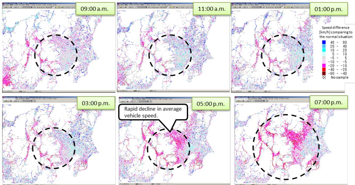
**Figure5 –Speed difference of Traffic Scope on the heavy snow day**
