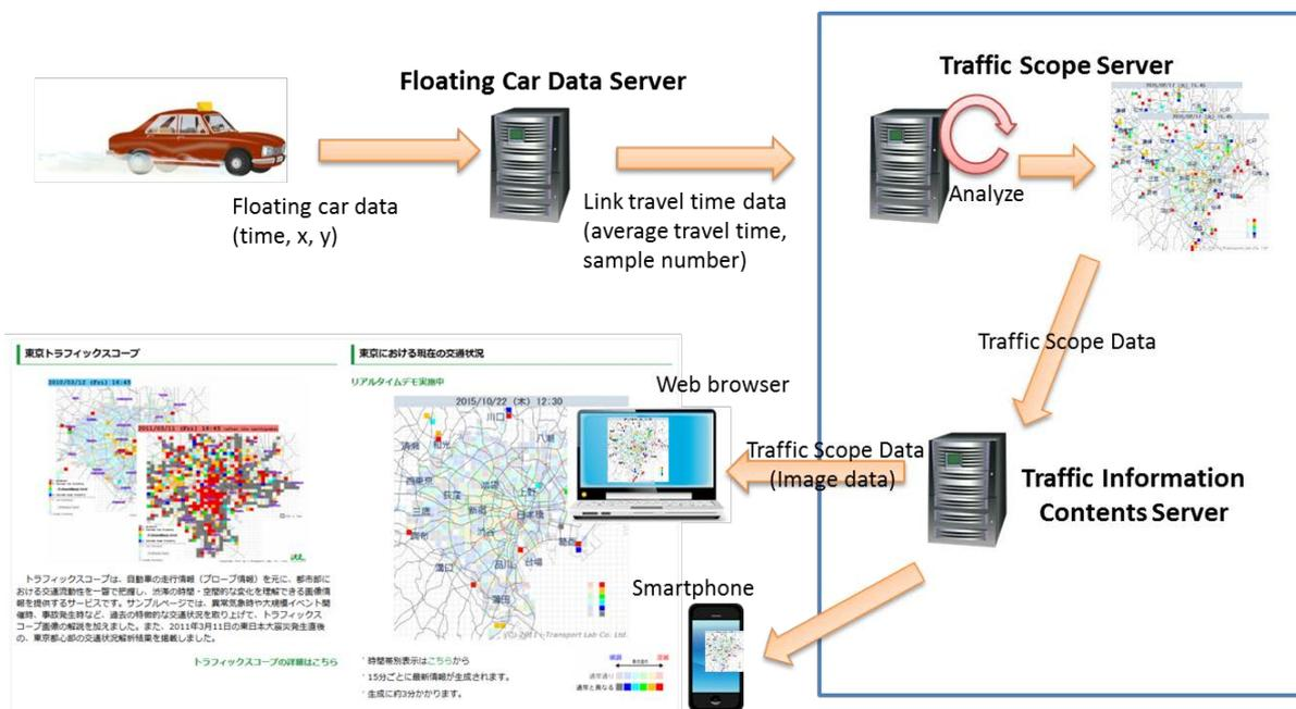
**Figure2 – System image of Traffic Scope system**
